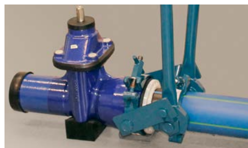
8. Insert the pipe through the NOVO-Grip® III ring into the socket until it rests concentrically against the sealing gasket. Avoid deflection during assembly.
