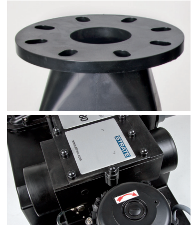
The STRATE AWALIFT 80 has a DN 80 / 100 flange connection to the pressure line which can be used without an adapter for both sizes, as well as two DN 100 inlets.
