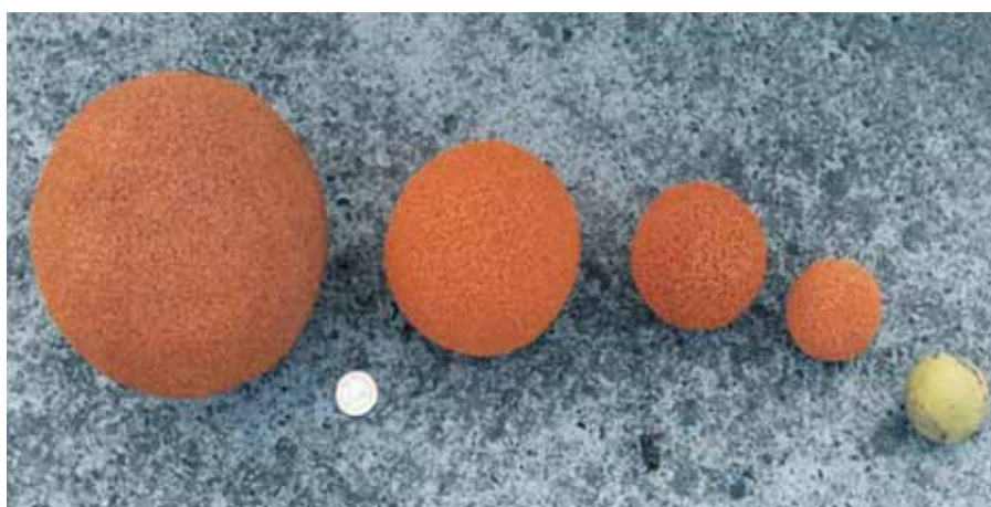
Cleaning pigs of different sizes (source: Dipl.-Ing. M. Mäding)
